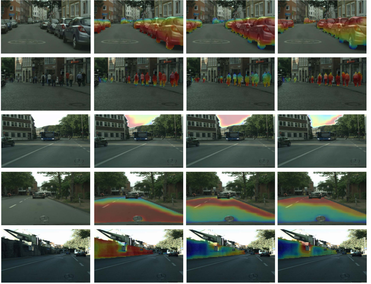
Fig. 7. Activation map of multi-prototypes. The leftmost column is the input image, and the images in columns 2 to 4 correspond to three different prototypes of the category, respectively. The categories shown from the top to the bottom are car , person , sky , road and wall .
